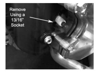
4. Install the plug into cylinder head and torque to 20ft.-lbs. Be careful not to overtighten the spark plug.
