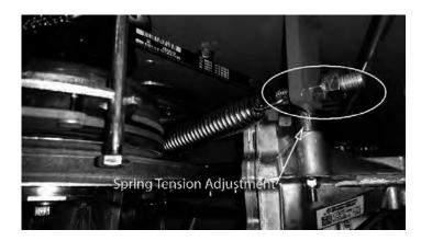
Use a belt tension gauge to ensure the proper tension. Your dealer or service center will have a belt tension gauge or you can buy one (Part Number 041-9999-00).
