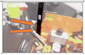
• Remove and retain the two nuts that secure the bottom portion of the ROPS tube.
