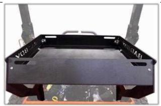
When all of the bolts are in place, adjust for square and level and tighten all of the bolts.
