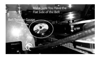
Use a belt tension gauge to unsure the proper tension. Your or service center will have a belt tension gauge or you can buy one (Part Number 041-9999-00).
