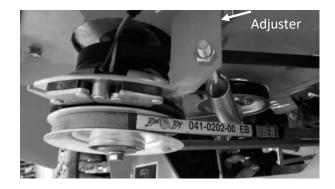
The tension should be adjusted so that there is between 60 to 65 lbs. of tension on the belt. This can be checked with a belt tension gauge as shown to the right.
