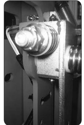
The control arm blocks have grease fittings located on the top and bottom of each block. Grease one time a year.
