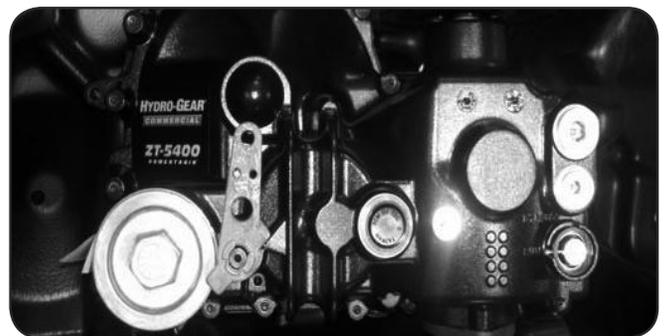
Filter housing cap. (do not over tighten)
