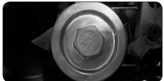
The check plug is located at the top center of the inside case of each transaxle. The transaxle can be filled with oil by removing these check plugs from both transaxles and pouring the oil in the hydro overflow tank, located behind the seat. Oil will begin to run out of the check plug holes when the transaxles are full. Use only 20w50 motor oil in the hydro system.
