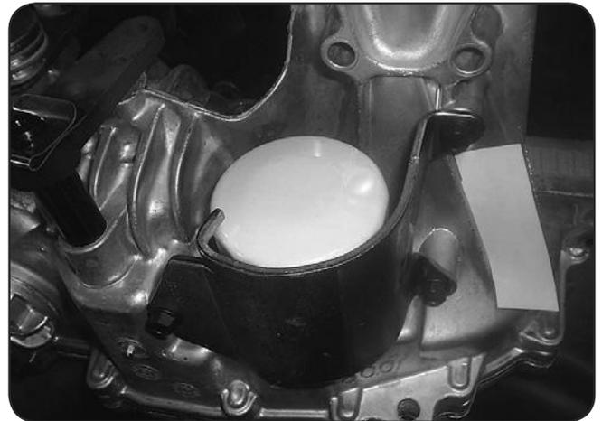
Shown right is the CZT transaxle. The large cap on the lower left is the filter housing cap.
