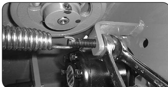
Tightening the two  $\frac{3}{4}$ " jam nuts on the right side will increase the belt tension on all models. Factory setting is about .030" (about the thickness of a credit card) between coils as shown.
