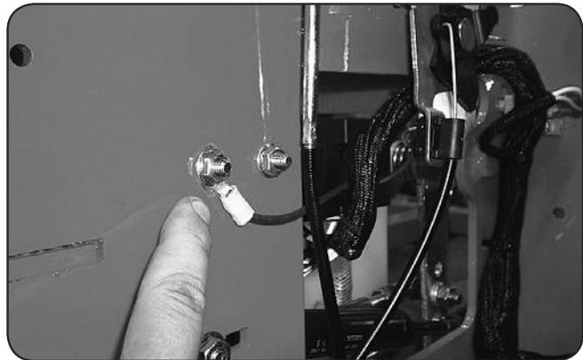
Check the condition and connection of the relays located under the seat. Ensure that they are clean and connected. Make sure that wire terminal ends have not been pushed out of the relay block.
