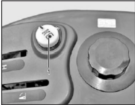
(1) PTO ON/OFF Switch
