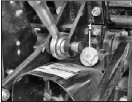
(1) Transmission Fluid Filler Hole
