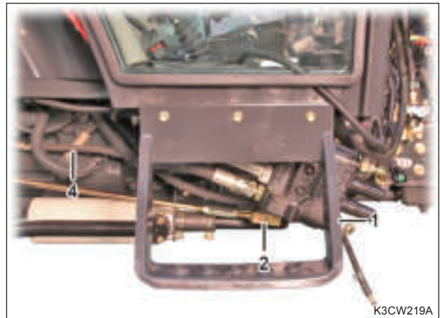
10. Remove the 4WD lever (1) and range shift lever (2) from the lower left section of the cabin.
