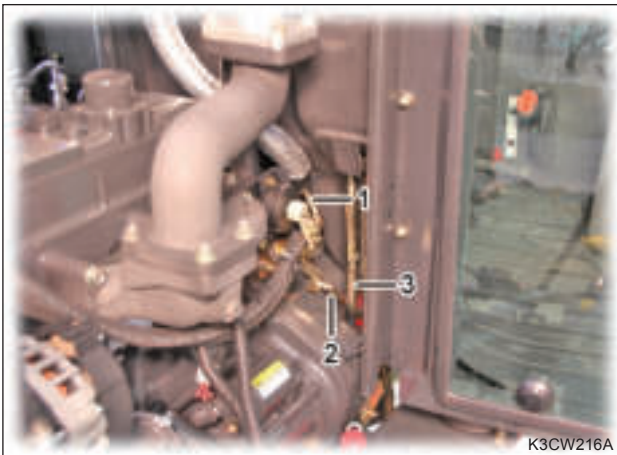
8. Disconnect the fuel supply hose (1) and fuel return hose (2) from the right side of the tractor.
