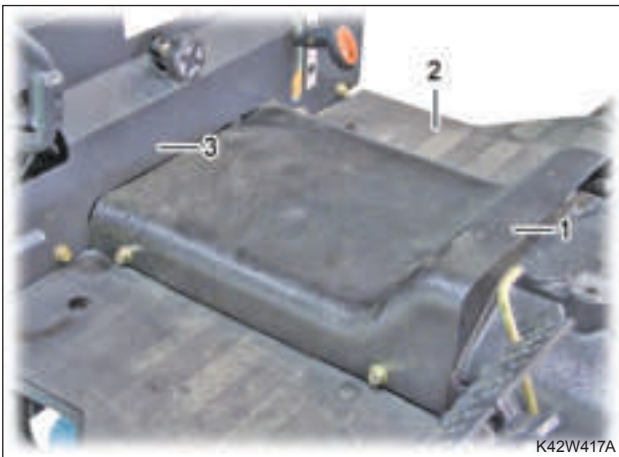
7. Remove the transmission case cover (1), floor mat (2)(LH, RH), dust cover assembly (3).
