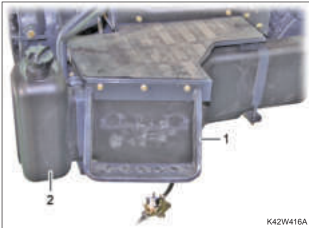
6. Remove the footstep (1) and fuel tank (2).
