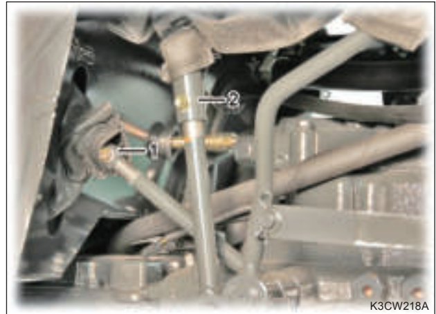
10. Remove the 4WD lever (1) and range shift lever (2) from the lower left section of the cabin.
