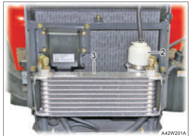
8. Remove the air cleaner (1) and reservoir tank (2). Remove the oil cooler(3).
