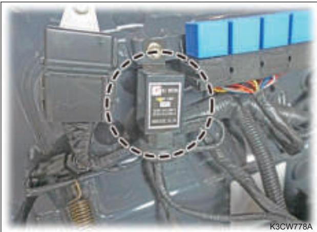
The flasher unit is installed on the upper left side of the dash panel.
