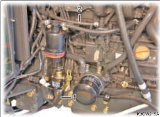
8. Disconnect the fuel supply hose (1) and fuel return hose (2) from the right side of the tractor.
