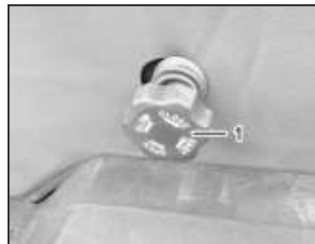
(1) Flow Control Valve
