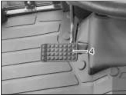
(1) Brake pedal (free play: 5 - 10 mm)
